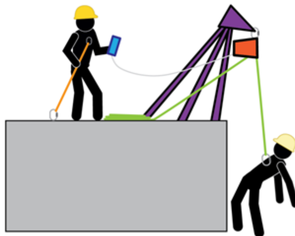
Figure 5. An illustrative example of a complex Remote Rescue using a remotely operated winch
